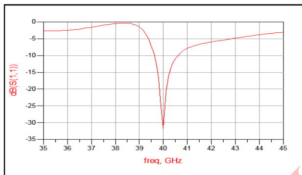
Fig.11 Return loss Vs frequency at 40GHz of receiver system
