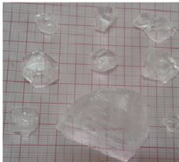
FIGURE 2. Photograph of as grown TGS mixed ADP (9:1) Single crystals
