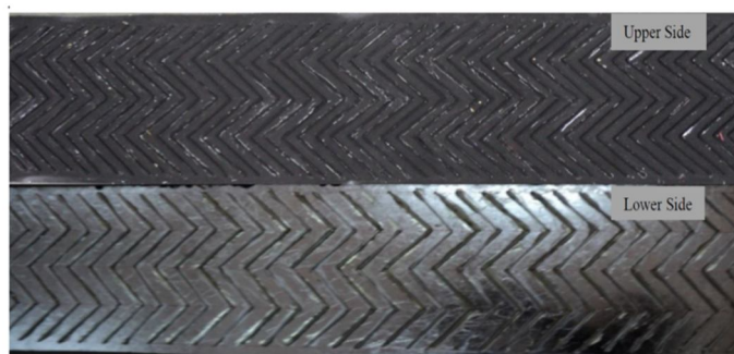
Fig 2.6 pictorial view of W-shaped roughness geometry on absorber plate.
