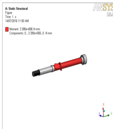
Fig:7. Moment applied on shaft
