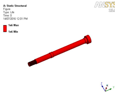
Figure: 13. Life cycle of modified shaft
