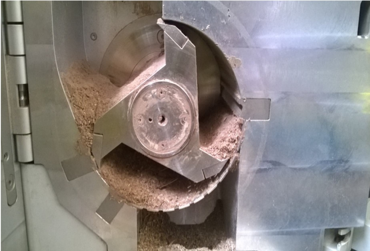
Fig- Miller set at 700 rpm with 4mm sieve
