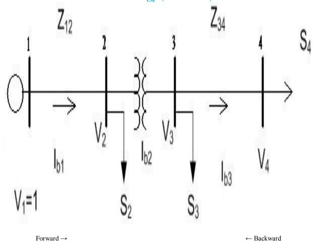
Fig. 1. Radial Distribution System
