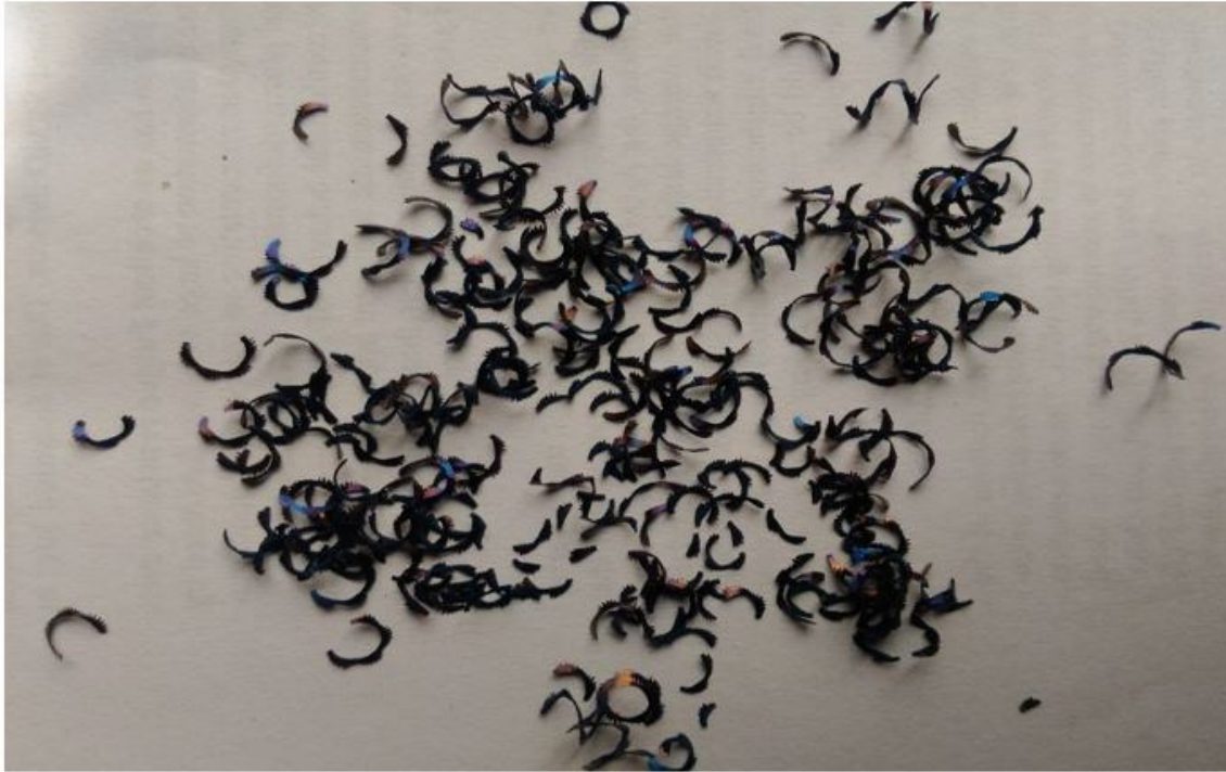
Fig 16: Discontinuous chips for DCT tool inserts
