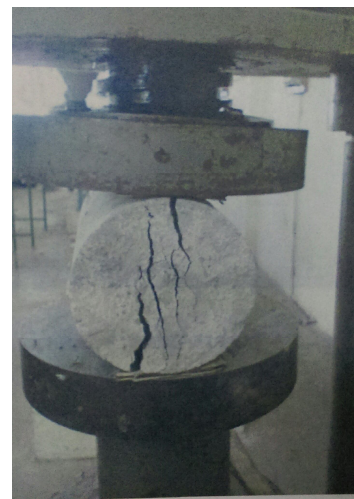
Fig 4 Tensile strength Test
