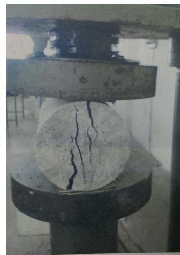
Fig 4 Tensile strength Test
