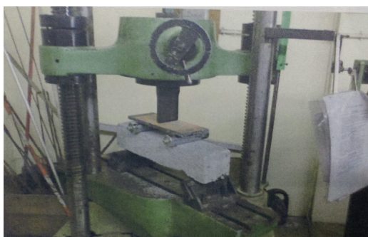
Fig 6 Flexural Strength Test
