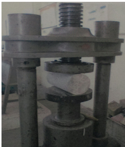
Fig 3 Tensile strength Test
