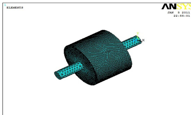
Fig.6 Three-Dimensional Finite Element Model Of Roller Assembly
