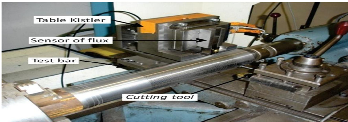
Fig. 1. Cutting test and machining on an instrumented Gazeneuve lathe installation
