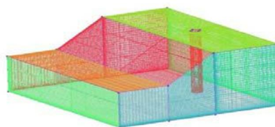
Figure.3. Meshed fuel tank used in simulation
