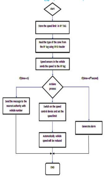
Initially in the RF tag the speed limit of the vehicle will be set. Along with this, it also contains the type of zone. The RF tag will be placed near the safe zones.
