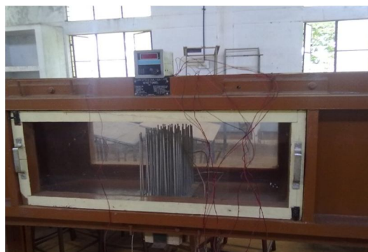
Fig.2: Model Setup inside the Wind Tunnel
