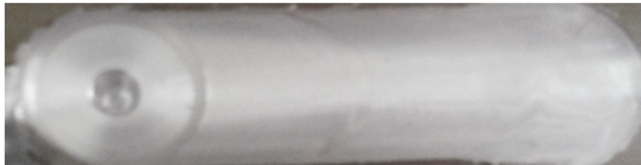
Fig 2 Surface morphologies of weld without defects
