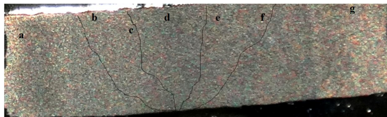
Fig 3 Macrostructure conical threaded pin
