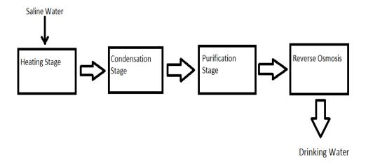
Fig. 1 Process blockdiagram
