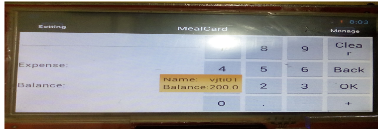
Figure IV: The information in card displayed as card is kept on RF reader.
