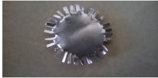
Fig 2 fabricated serrated fin with above dimensions.
