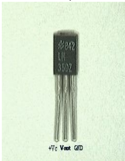
Figure 4 Temperature sensor device
