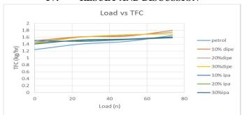
This graph shows the TFC of the all the samples and petrol, almost all the blends has more TFC. On comparison the sample containing 30% of Iso Propyl Alcohol is comparatively good.
