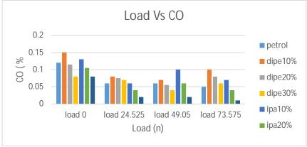
This graph shows the CO emission of the all the samples and petrol, almost all the blends have more emission on initial stage and on applying load the emission comparatively the alternative blends has very low emission. On comparison 30% of Iso Propyl Alcohol
