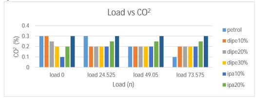
This graph shows the CO<sup>2</sup> emission of the all the samples and petrol, almost all the blends has more emission when compared to petrol and on applying maximum load the petrol has very low emission. On comparison all are mostly equal and more than petrol.
