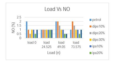
This graph shows the NO emission of the all the samples and petrol, almost all the alternative blends has very low emission. On comparison all are mostly same and less than petrol. On comparison 20% Iso Propyl Alcohol is comparatively good.
