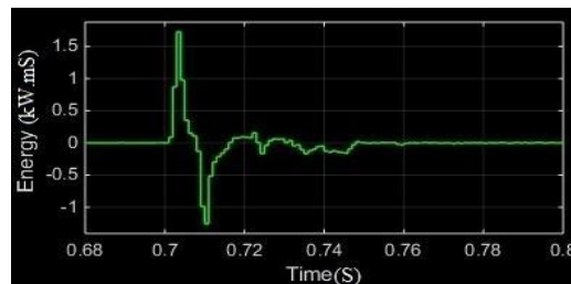
Fig.10. Transient energy during rectifier fault
