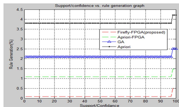
Figure 3: Comparison between Apriori, GA, Apriori + FPGA and Firefly+FPGA for the Rule generation ratio for support/confidence
