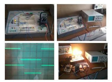
Circuit connection of ZCD and its output are shown in this image. The output is shown on a CRO. Two waveforms are shown by CRO one is current waveform and other is voltage waveform.
