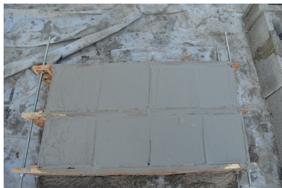
Fig.3 Casting of Specimen
