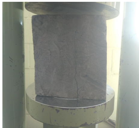
Fig.6 Compressive Strength Test
