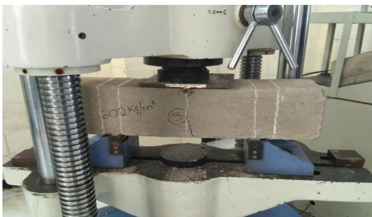
Fig.8 Flexure test setup
