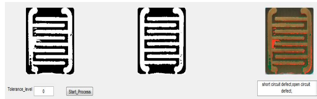
Fig. 6 GUI for fault detection
