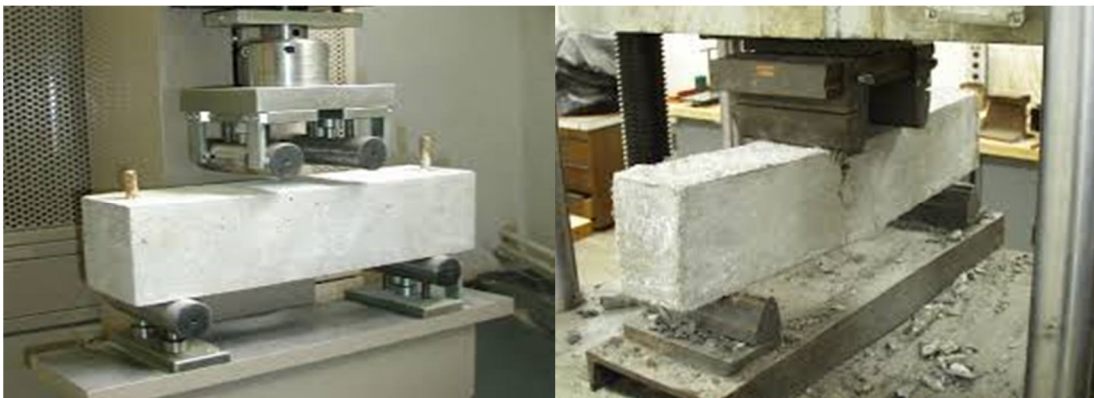
Fig 3.9 Flexural strength setup before testing
