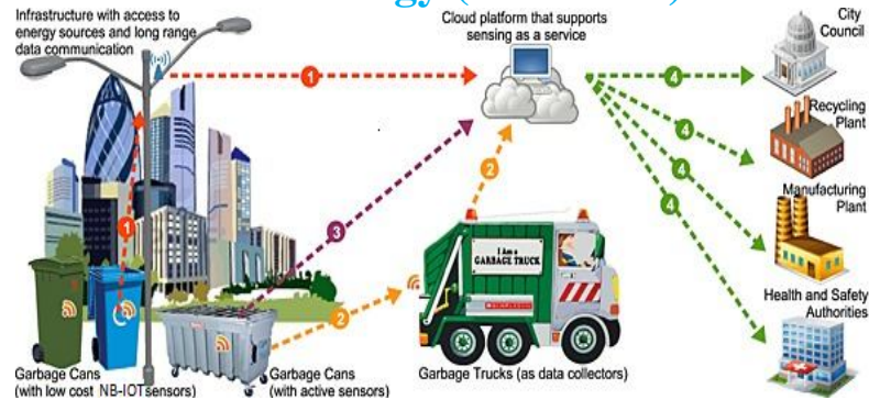
Fig 8: Smart waste management based on NB-IOT.
