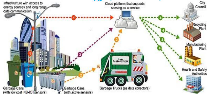
Fig 8: Smart waste management based on NB-IOT.
