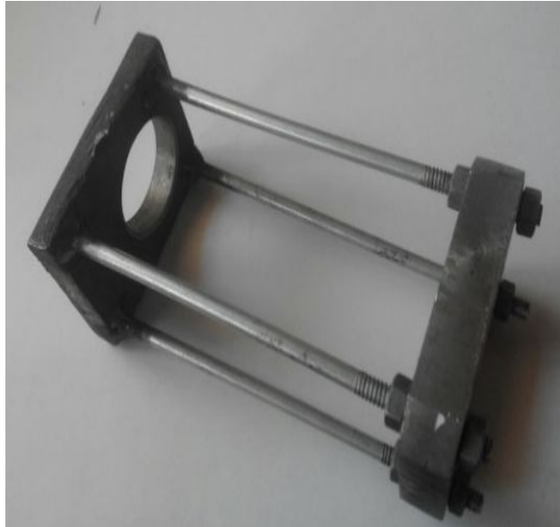
Fig.4.2 image of bracket and supporting members fabricated.
