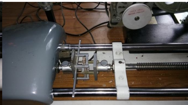
Fig.9 Sample loaded condition for flexural testing
