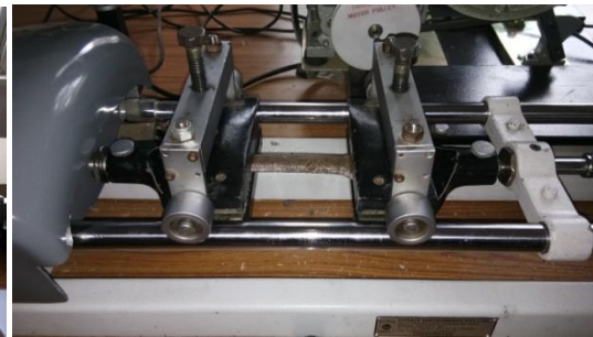
Fig.7 sample loaded in Tensometer
