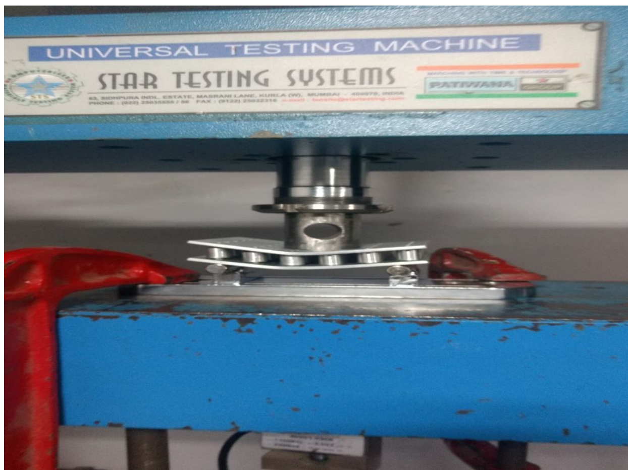
Fig.6-Bending Test on Sandwich Structure
