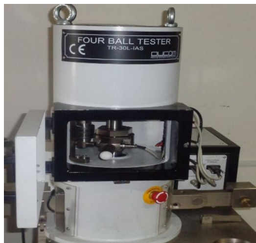
Fig.5 : Four ball tester test section ,mfg.by Ducom,Bangalor,India.
