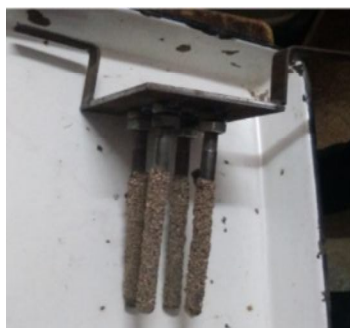
Fig.3 Four Pile Group
