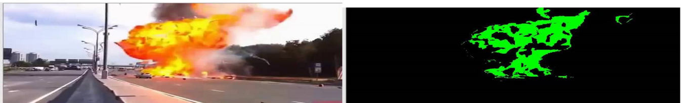
Figure 5.1 (a) shows the original frame i.e frame1, the Figure 5.1 (b) which is the result of the Fire detected image
