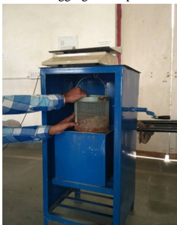
Fig. 3 Wire bucket for Specific gravity
