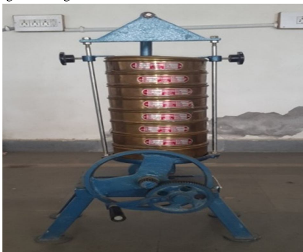
Fig 1 Sieve shaker with sets of sieve
