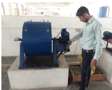
Fig. 4 Los angeles abrasion testing machine
