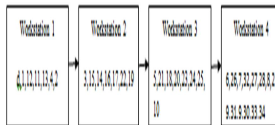
Figure 2 Configuration of assembly line as per RPW technique
