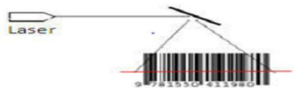
Fig2: Working of Barcode
