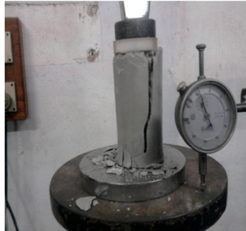
Fig: UCS test on wax coated Lime treated fly ash
