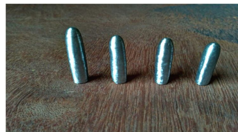
Fig 2: wear test pins extracted from hardfaced plate
