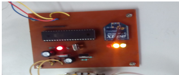
Fig 3: Electronic circuit for Transmitter section
