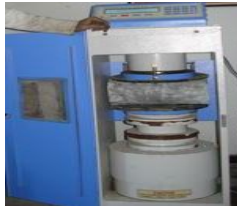
Fig.5 split tensile strength testing
