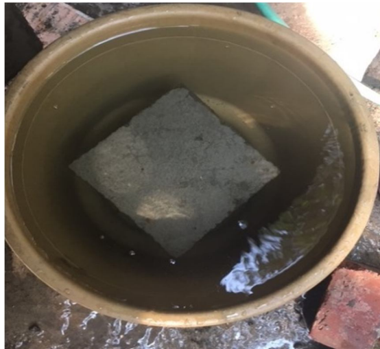
Figure no 1:- cube submerged in a bucket full of water.
