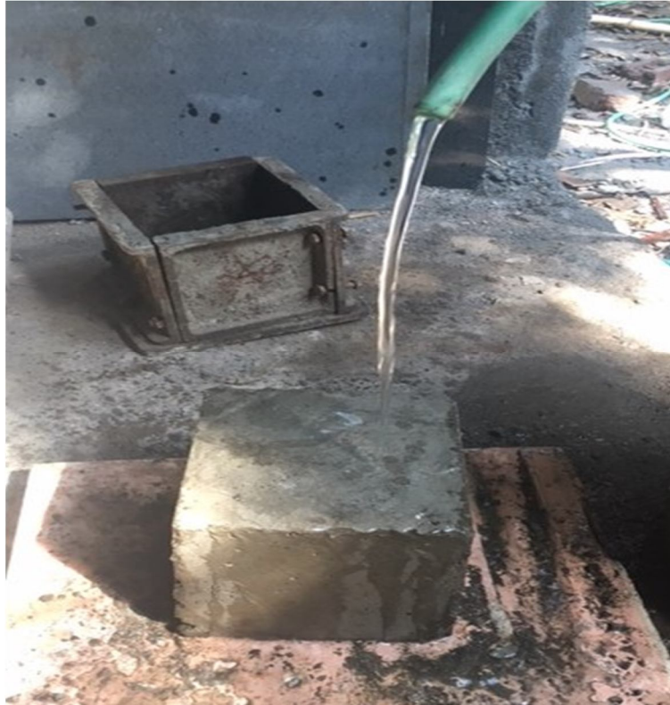
Figure no 2:- Spraying on a concrete cube.
