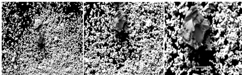
Fig. 4 SEM images of 1.5% Eu doped YGdB 2 O 6 phosphor
