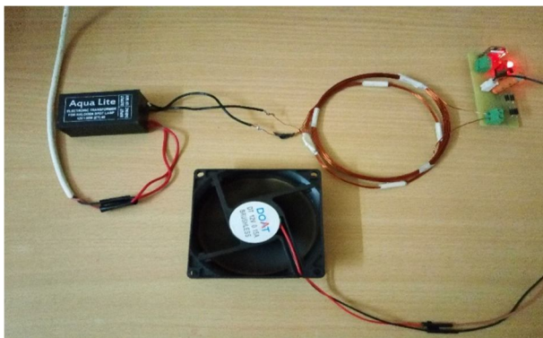
Fig. 3 Wireless Power Transfer for Fan
