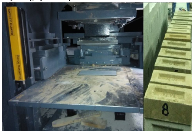
Fig.3 Casting of block in Hydraulic Compression Machine and Sample
