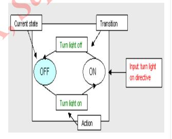
Moore Machines -- Outputs can be determined by the present state alone, or by the present state and the present inputs, ie outputs are produced as the machine makes a transition from one state to another.
