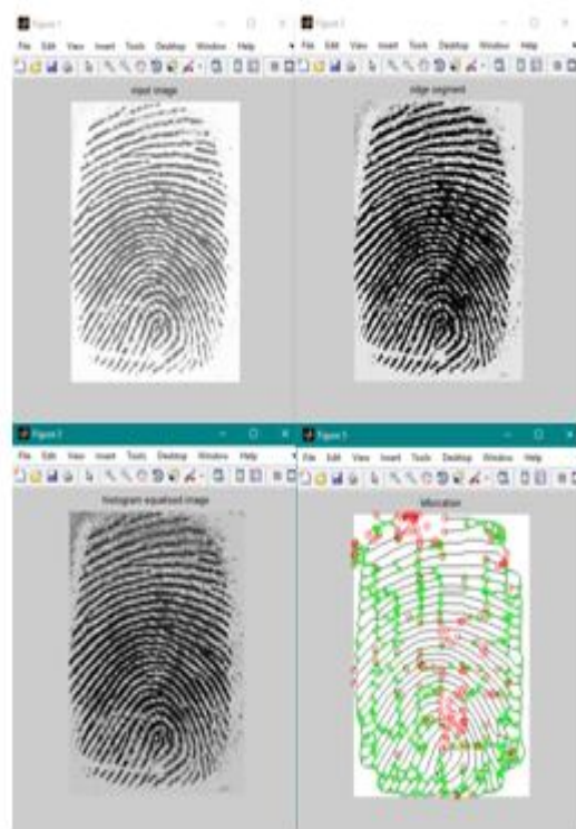
Fig.3. (a) Input image (b) Ridge segment (c) Histogram equalization (d) Bifurcations
