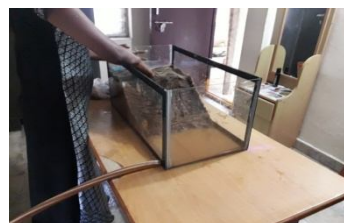
Fig.5: Container with drain pipe for collecting runoff water
