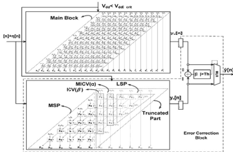
12x12 bit ANT multiplier is implemented with the six-bit fixed width replica redundancy block.
