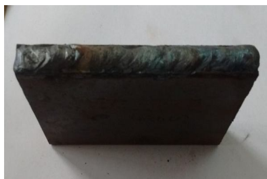
Fig. 2 Deposition of weld metal on base metal
