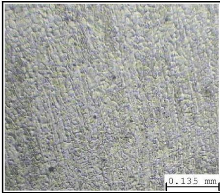
Fig. 10 Microstructure for E410 electrode weld metal
