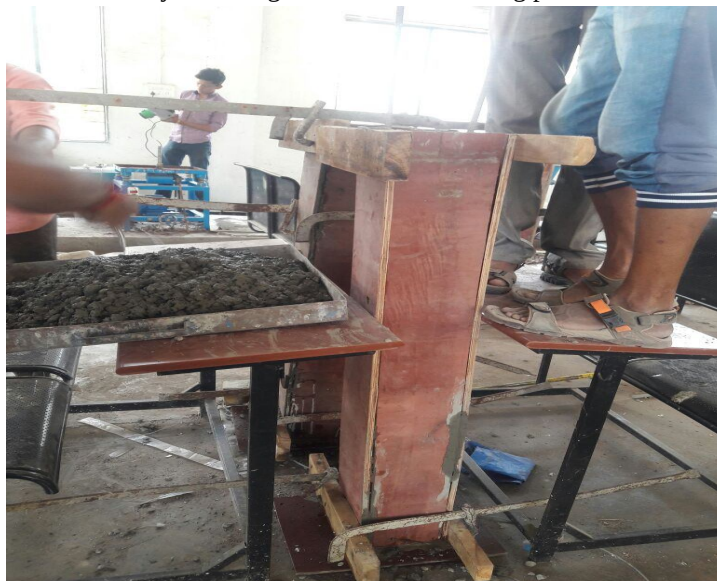
Figure 4: Mixing and Casting of RC Column Specimen
