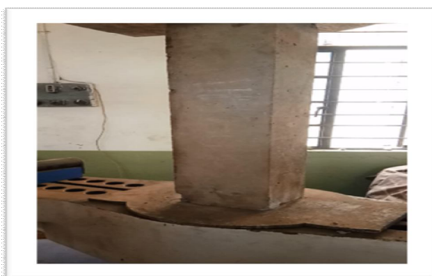
b) 700 mm column specimen tested on UTM
