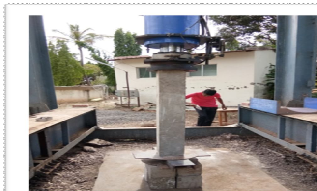
a) 1100 column specimen tested on Hydraulic loading frame
