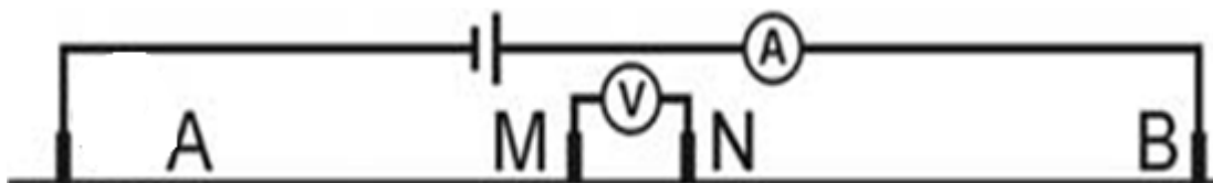
Fig.3: Schlumberger array configuration
